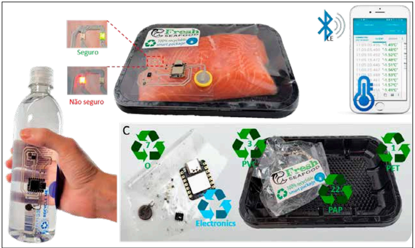
Recyclable printed circuits for continuous temperature monitoring of packages throughout the entire supply chain
