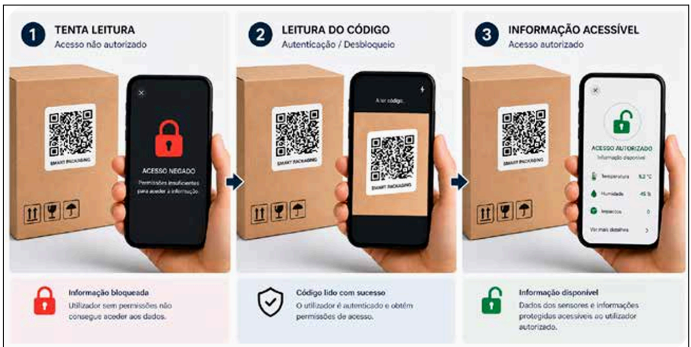
Sequence of interactions with the smart packaging: unauthorized access attempt, code scanning by an authorized user, and unlocking of the information after authentication.
