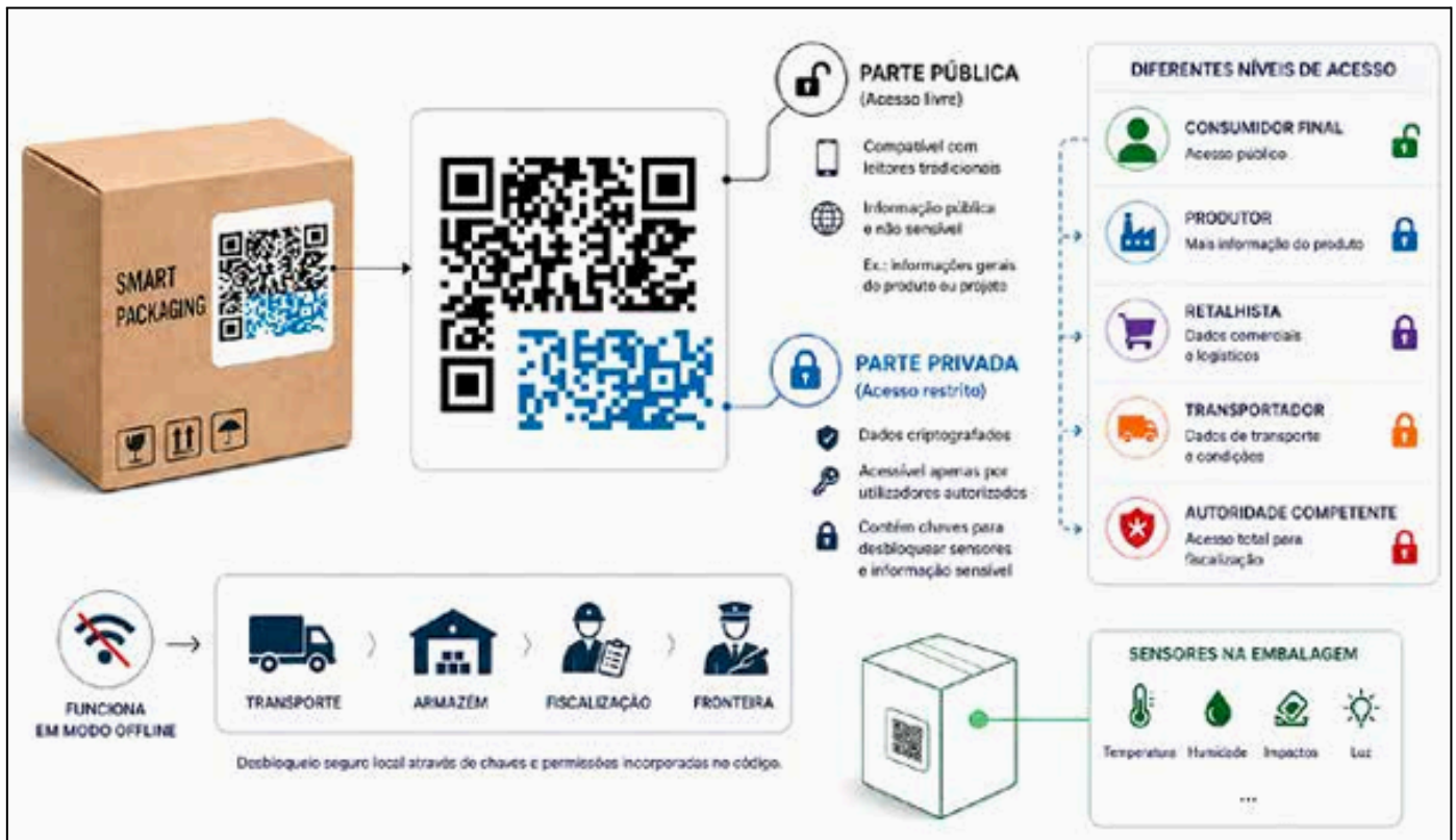
A hybrid barcode applied to smart packaging, combining a public component compatible with conventional scanners and an encrypted private component for secure access to information.
